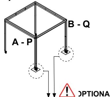
**STAFFA REMOVIBILE PER POSIZIONAMENTO A TERRA STRUTTURA MOBILE / BEWEGLICHES PROFIL ZUR BEFESTIGUNG VON PFosten AM BODEN FÜR BEWEGLICHE PERGOLA / ÉQUERRE ENLEVABLE POUR POSITIONNER LA PERGOLA MOBILE AU SOL / BRACKET REMOVABLE TO PLACE THE MOBILE PERGOLA ON THE GROUND / ESTRIBO AMOVIBLE PARA POSICIONAR UNA PÉRGOLA MÓVIL**
